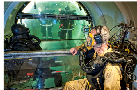
Figure 1: Four CUMA divers breathing trimix: 2 wet-working divers on underwater bicycle ergometers (electrically braked): 50 W, 5 min cycling; 5 min rest) wearing dry suits in 6-8°C water, one standby diver (partially wet, resting), and a team leader (dry, lightly working).
